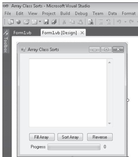
This form looks similar to the earlier projects in this chapter and features a test box for displaying array data. However, it also contains three buttons for manipulating large arrays and a progress bar object that gives the user feedback during longer array operations. (Visual feedback is useful when computations take longer than a few seconds to complete, and if you use this code to sort an array of 3,000 array elements, a slight delay is inevitable.)
