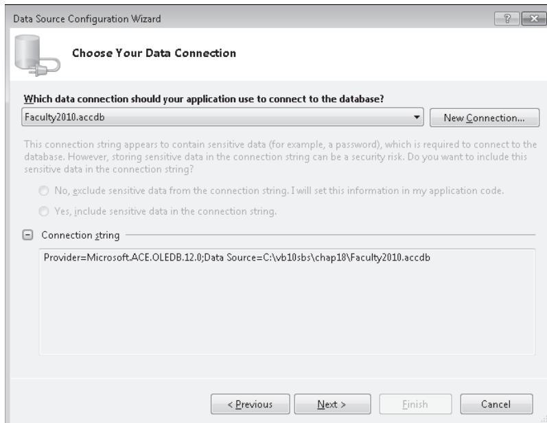
The connection string identifies a *provider* (also called a *managed provider*) named Microsoft.ACE.OLEDB.12.0, which is an underlying database component that understands how to connect to a database and extract data from it. The two most popular providers offered by Visual Studio are Microsoft OLE DB and SQL Server, but third-party providers are available for many of the other popular database formats.
